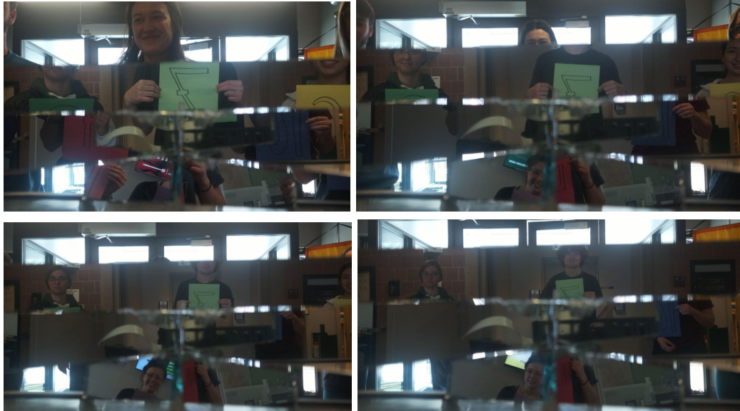
Figure 5. The unprojected images acquired during the testing of the PanLapse Device, with the smallest radius from the device in the top left corner and the largest radius in the bottom right. (Photo Credit: N. Heronema)
