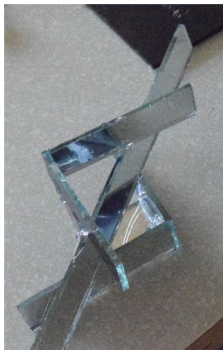
Figure 2. The mirror array utilized within the PanLapse device, prior to vertical angle changes. (Photo Credit: N. Heronema)
