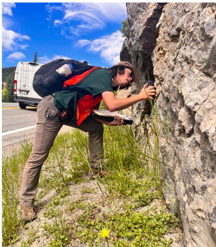
Adam Rang measures the strike and dip of a fault found in a road cut outside of Silverton, Colorado. Photo by Madeline Ferguson
