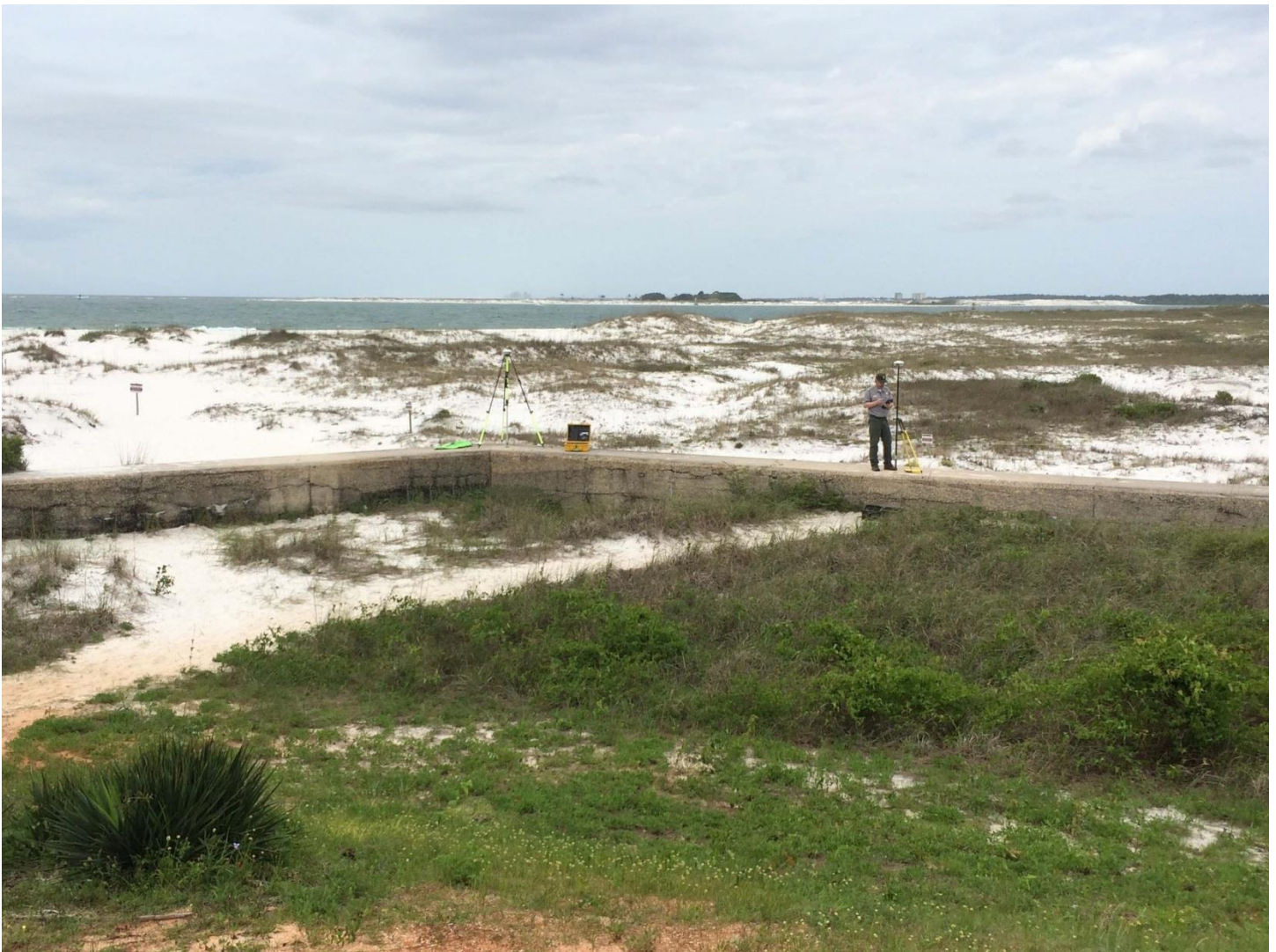
Collecting precise elevation data at Fort Pickens, Gulf Islands National Seashore, Florida for sea level rise vulnerability analysis and park planning
