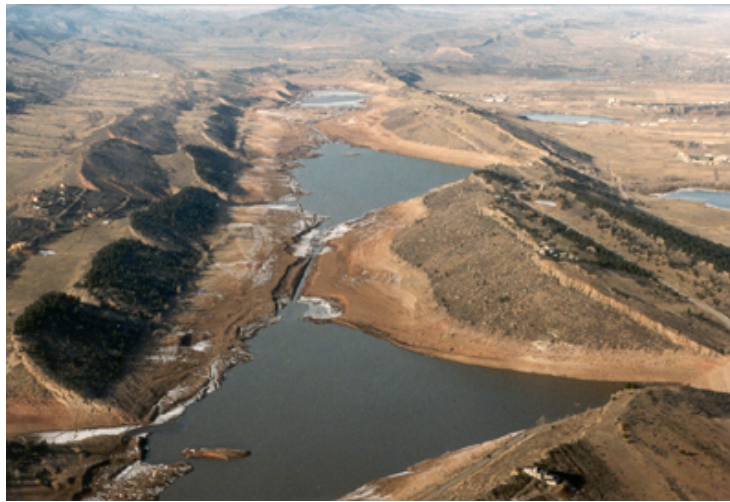
Figure 3. Horsetooth Reservoir during the drawdown (photo: Ben Alexander). The view is to the north, with Spring Canyon pool in the foreground connected to Dixon pool by a trench. A trench also connected Dixon and Soldier Canyon pools, with Soldier Canyon at the top of the image.
