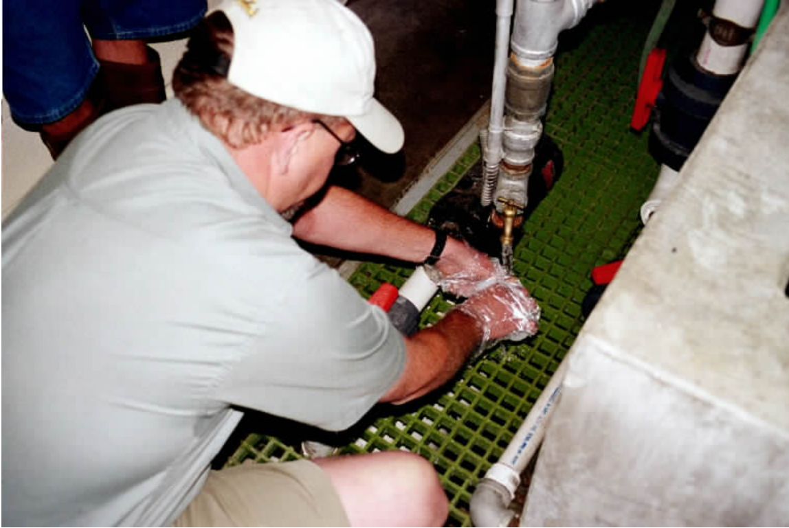
Figure A4.3. Water was collected using clean techniques. In some instances, hatcheries used multiple water sources and samples were collected after they had been thoroughly mixed prior to entering raceways, as shown above (photo: P. J. Martinez).
